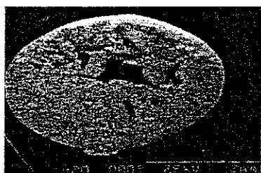
Figure 3. Cross-section of Bio-Sep ® bead.
