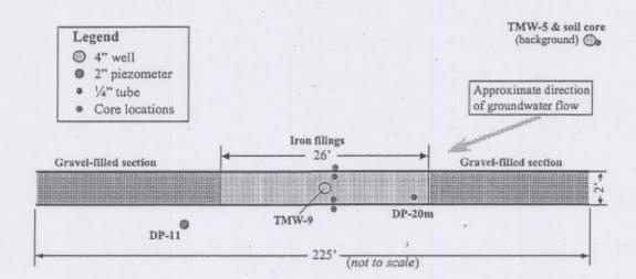
Figure 1. Schematic drawing of the iron/gravel barrier at the Oak Ridge Y-12 Plant site and the locations of groundwater sampling wells and soil/iron cores used for the determination of microbial population and community structure.
