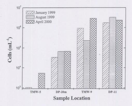
Figure 2. Microbial population or abundance biomass by PLFA analysis in groundwater from monitoring wells located at the upgradient soil (TMW-5), within the Fe<sup>0</sup> barrier (DP-20m and TMW-9), and at the downgradient soil (DP-11).
