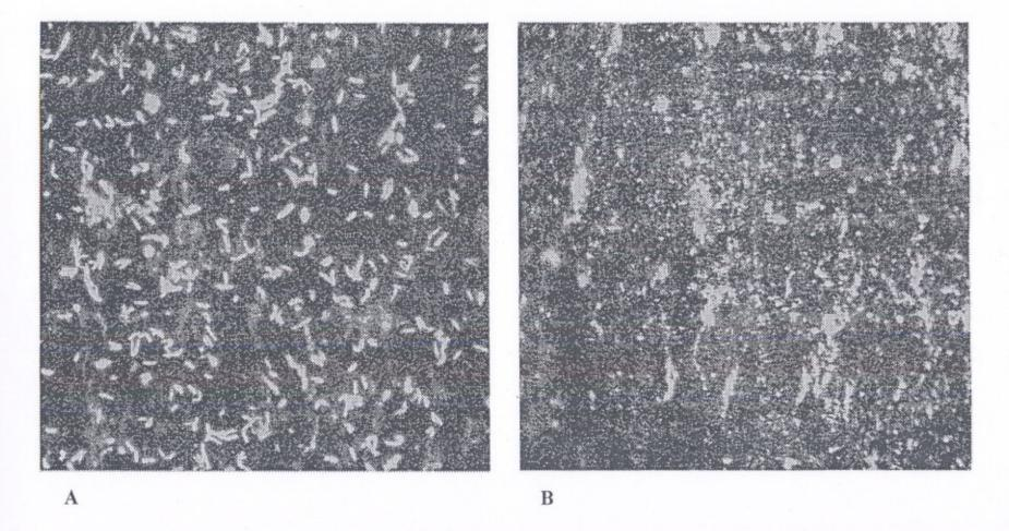
Effect of wiping Aluminium 6061 on which *Mycobacterium pflei* containing green fluorescent protein had been air dried. Surface was wiped Kimwipe in two dimensions with a solvent of 70% aqueous alcohol. A. Before wiping. B. After Wiping. Taken with a confocal microscope and detected by fluorescence (excitation ~395nm, emission ~509nm) The horizontal field is ~220 um long.
