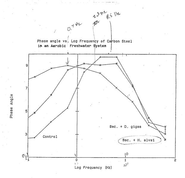
Figure 4. Phase angle versus the log frequency in the EIS analysis of the systems used in Figure 3. The triculture of <a href="Bacillus sp. + H. alvei + D. gigas">Bacillus sp. + H. alvei + D. gigas</a> (crosses), biculture of <a href="Bacillus sp. + H. alvei">Bacillus sp. + H. alvei</a> (open squares), and sterile control (x) are indicated. The shift to lower frequencies (to the left) may indicate possibly greater localized activity.
