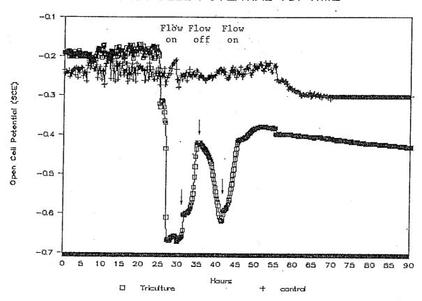
Figure 2. Open cell potential trace of the control (without microbes) (crosses) and the triculture consisting off the <u>Bacillus sp. + H. alvei + D. gigas</u> (open squares) against the calomel electrode. The effects of the microbial biofilm (initial drop) and manipulations in stirring and flow rate are indicated in this aerobic freshwater system.
