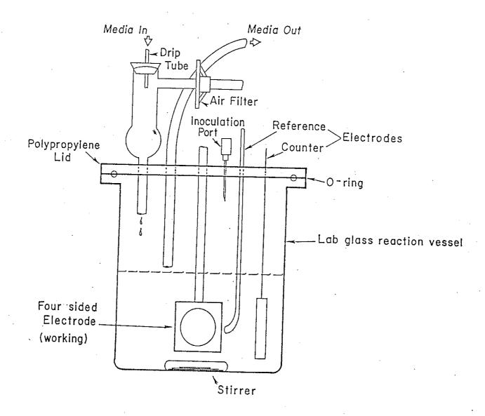
Figure 1. Experimental test vessel for the electrochemical analysis of corrosion by various combinations of monocultures. Both the media in and media out are connected to reservoirs with masterflex pumps and silastic tubing. The four-sided electrode can be rotated so each face of the working electrode can be placed adjacent to the reference electrode during the electrochemical analysis.
