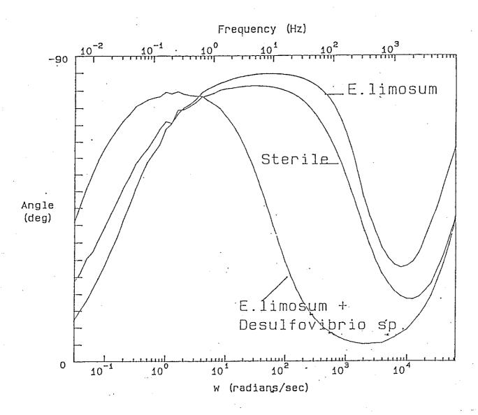
Figure 6. Phase angle versus the log frequency in the EIS analysis of the experiment illustrated in Figure 5. The biculture of  $\underline{E}$ .  $\underline{limosum} + \underline{D}$ .  $\underline{desulfuricans}$  showed the most pronounced shift in maximum phase angle at lower frequencies (left) which may indicate more localization of the MIC activities.
