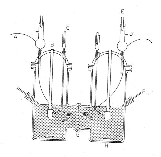
FIGURE 5. Dual chamber, continuous flow apparatus for comparison of MIC and control corrosion parameters. A - common electrode (titanium), B - working electrode, C - Luggin probe, D,E - drip tube for media input, F - media outlet, G - teflon membrane 0.2  $\mu$ m pore size, H - magnetic stirrer.
