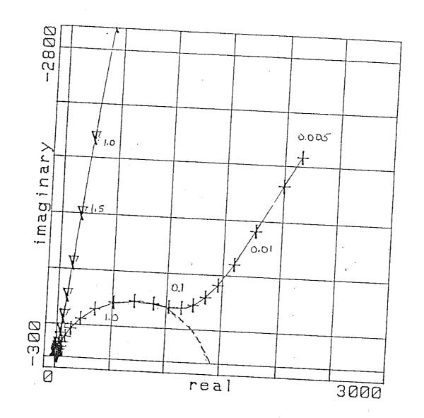
FIGURE 3. Nyquist complex plane plots of electrochemical impedance spectroscopy of AISI 316L stainless steel exposed to diluted nutrient medium in seawater for 12 days. ( ) indicates the sterile control, (+) inoculated with a consortium of microbes from a black marine sediment. Numbers indicate the sinusoidal sweep frequency in KHz. Low sweep frequencies show anomalous behavior related partly to localized corrosion. Data from (9).
