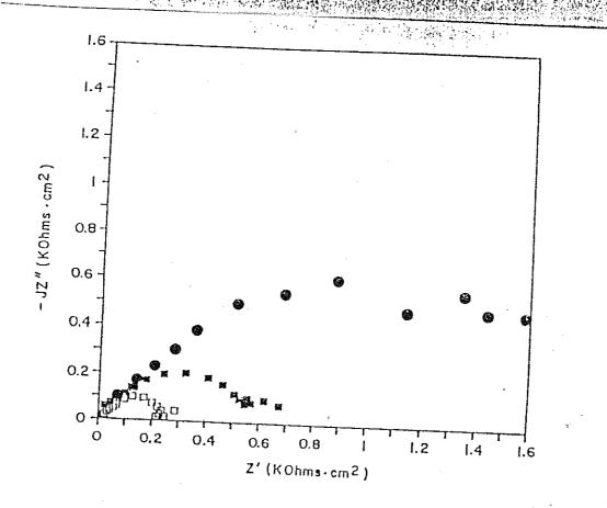
FIGURE 2. Nyquist complex plane plot of electrochemical impedance spectroscopy of mild steel (C1020) coupons incubated in artificial seawater to which nutrients had been added. Middle curve ( ) shows initial response; lower curve ( ) shows response after growth of vibrio natriegens for 4 days and the uninoculated control after 4 days. ( ) showing passivation when compared to the initial value. Note the "second loop" in the low frequency end of the plot. Data from (7).
