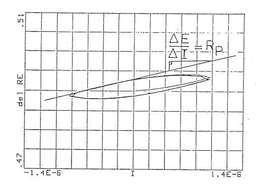
FIGURE 1. Small angle cyclic voltametry of AISI 316L stainless steel incubated in seawater enriched with diluted media. Showing the hysteresis induced in part by the capacitive component and the tangents used to determine  $R_{\rm p}$ .
